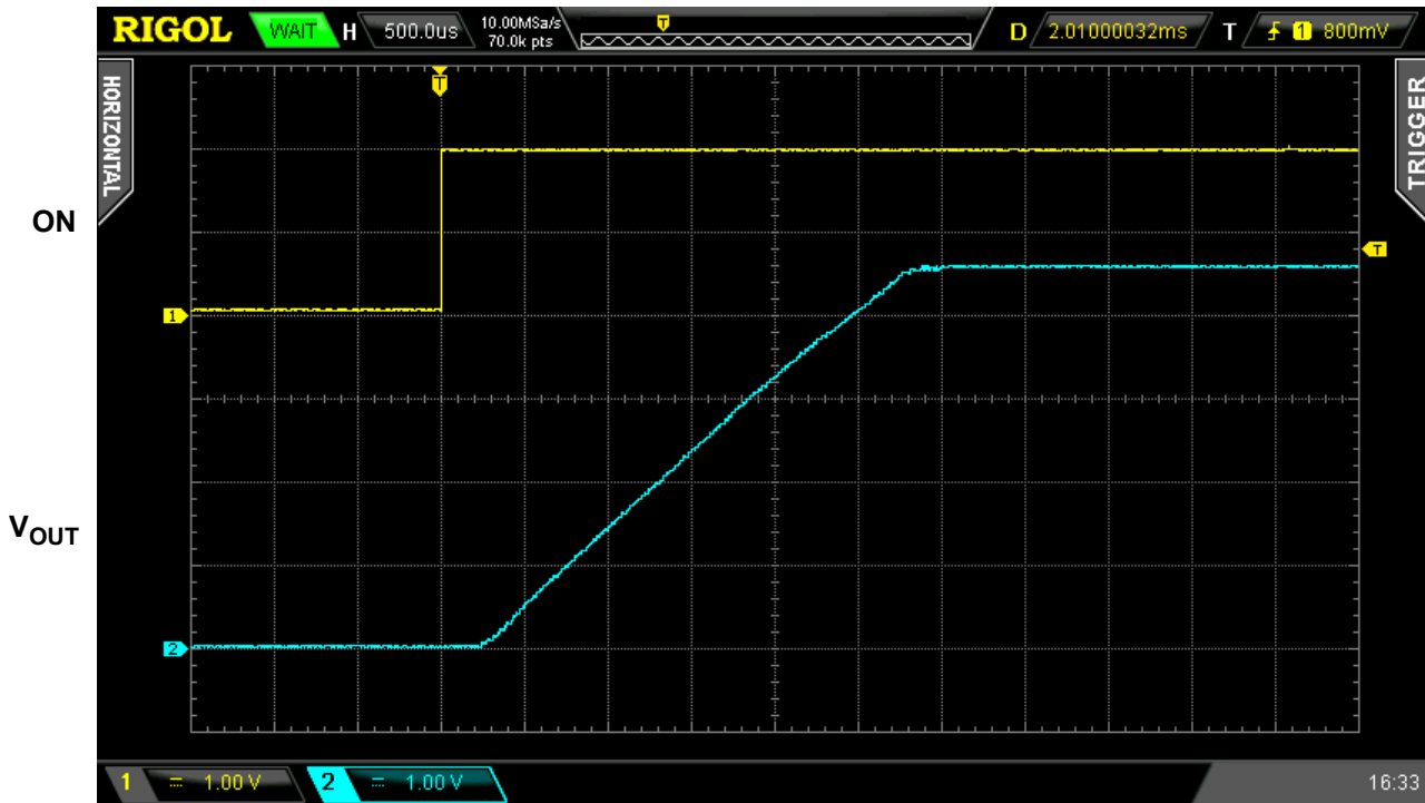
Figure 2. Typical Turn ON operation waveform for V_{IN} = 4.5\text{ V} , C_{SLEW} = 18\text{ nF} , C_{LOAD} = 10\text{ }\mu\text{F} , R_{LOAD} = 100\text{ }\Omega
